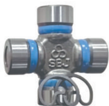
Uj Cross Suitable For Mini With Outer Locks (30x82mm) Part No. NR 517
